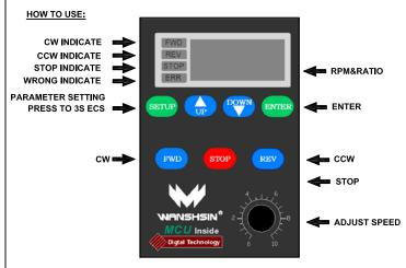
Pay attention: It will work under the digital display speed controller control mode. Please make the operation control mode to the digital display speed controller control mode.
